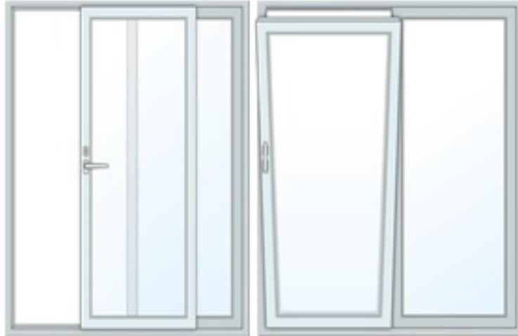
Tilt and slide doors are like a hinge door and a sliding door. They tilt into the room and then slide. The benefits of tilt and slide doors are better seals and the flexibility of sliding or tilting. You will need a retractable flyscreen door by another supplier.
