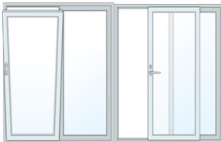
Tilt and slide windows have the benefits of a hinge window and a sliding window. They tilt into the room and then slide. The benefits of tilt and slide windows are better seals and the flexibility of sliding or tilting.
