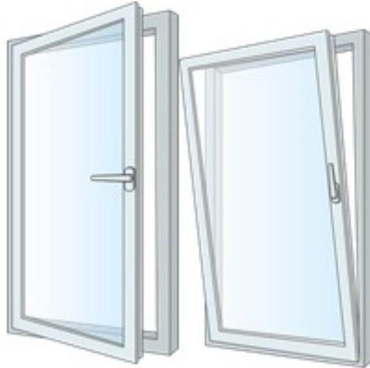
Tilt and turn windows are very popular in Europe and have the benefit of a multiple opening function and the seal very well. They can be locked in the open position and are perfect for evaporative cooling systems. They do open internally and you will need to be more creative with your window coverings.
