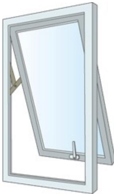
Awning windows have a hinge at the top and can wind out or be pushed out – depending on the supplier. They are good for cross flow ventilation and they seal very well. In terms of getting a big breeze in, they are not as good as some of the other styles.
